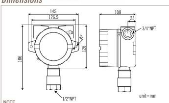
The picture and dimensions is for Explosion type A (Certificate on Housing only). Type B & C (EC-type) is on request.
