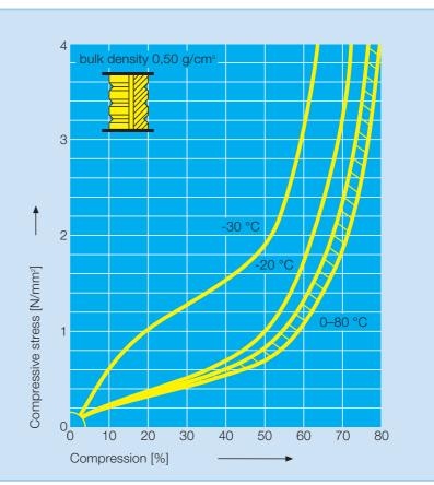
$\triangle$  Characteristic curves as a function of temperature
