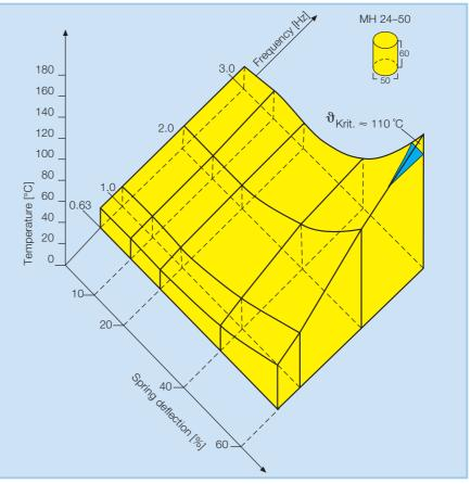
$\bigtriangleup$  Temperature increase caused by damping
